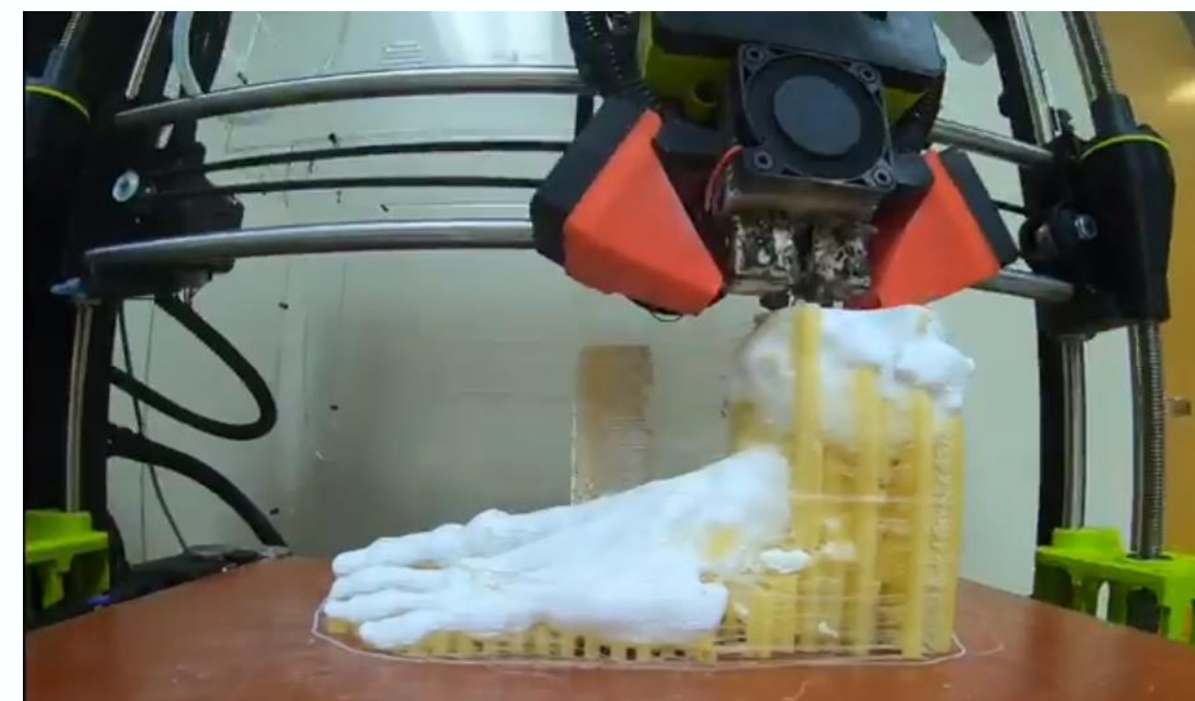
Figure 3. 3-D printing of reconstructed anatomical foot and ankle model.
