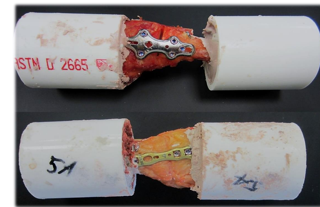
Figure 3. Specimens potted in 1.5 inch PVC pipe with auto filler. Top construct is the five-hole stainless steel plating. Bottom construct is the five-hole titanium alloy. The three-screw constructs were potted in the same fashion.
